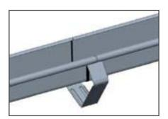
6. Attaching the box gutter connector: Hook the connector onto the bead at the front first, then pressing onto the adhesive surfaces of the seal throughout, wrap it around the gutter lengths over the join to the back.
