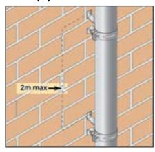
Downpipes should be installed using at least 2/no pipe clips per length. Mark out the clips locations and level with a sprit level or plumb line.
