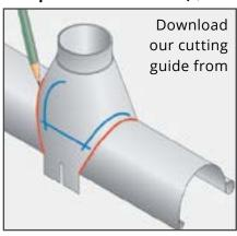
When installing a 'wrap around outlet' mark the desired location of the outlet by drawing a line either side of the outlet along its edge. Draw another line 20mm inside of the outer lines and join these
