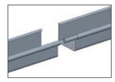
Insert the bead connector halfway into the front 'bead/ rolls' of both gutters, leaving an approx. 5 mm gap between the ends of the two gutter
