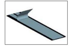
3. Remove the protection film from the adhesive surface (on ridged side) of the rubber sealing strip.
