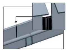
4. Attachthesealingstripoverboth ends of the gutters, starting at the 'bead/roll' at the front edge. Keep a slight tension on the strip to stretch round to the back while also smooothing/pressing down for a good bond.
