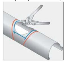
2. Use a hacksaw to make an initial hole in the gutter, and then use a set of tin snips to
