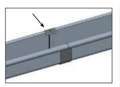
Finally fold the flaps at tehe back of the connector over the rear fold of the gutter lengths. TIP - Try to keep pressing down on the entire surface of the rubber seal (as much as possible) throughout to encourage a good bond over the entire length of each seal.
