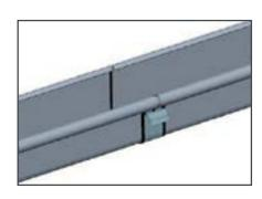
5. Remove the remaining protection film from the rubber sealing strip's final adhesive surface.
