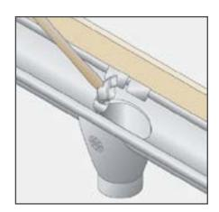
4. Tap the inner rough edges of the hole that was cut in the gutter, down into the outlet, to
