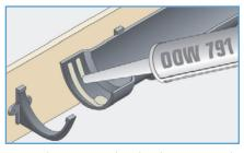
Apply two 6mm beads of DOW 791 silicone sealant either side of, and around the fixing hole.
