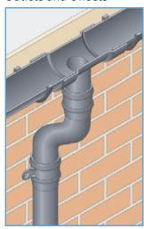
Commence installation from the gutter outlet by fitting offsets. Check vertical plumb line positioning and seal spigot and socket joints using DOW 791 silicone sealant.
