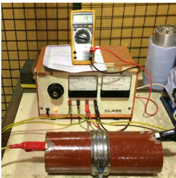
Electrical Continuity Testing
