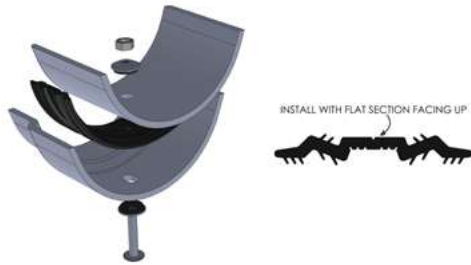
Fig 1. Illustration of how the specially designed & tested EPDM rubber strips seal the gutter lengths where they join.
